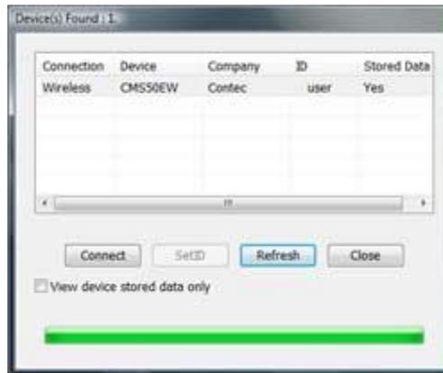
4. Check the "View device stored data only" box for downloading the stored data inside the oximeter. Then click the "Connect" button.
