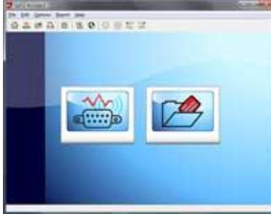
3. Select Connect Device button (the one that looks like a DB9 socket). A window would show the devices available (see diagram below).
