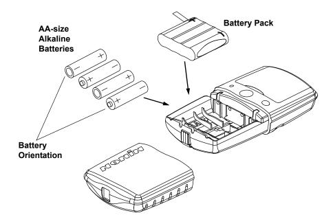
Figure 3: Installing Batteries
