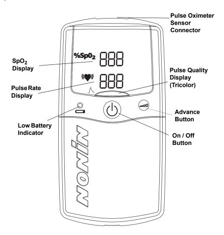
Figure 1: Displays, Indicators and Buttons
