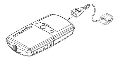
Figure 4: Connecting a Sensor
